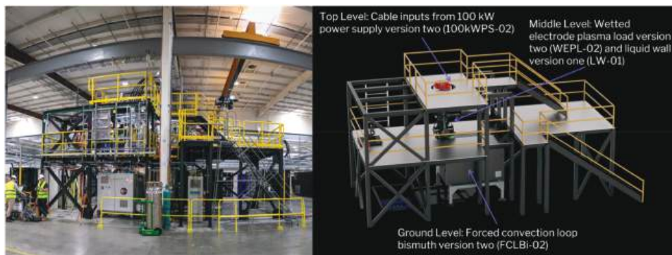
Fig. 3. Photograph of the Century platform in phase one configuration (left) and an illustration of major component locations (right).
