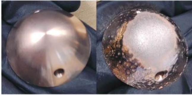
Fig. 13. SiMPL cathode nose cone tip inserts composed of tungsten-copper 10W3 (75% W/25% Cu) composite. Unused and pristine spare part, left. Identical unit after exposure to 50 repetitive high-power SFS Z-pinch plasma shots in SiMPL, right.
